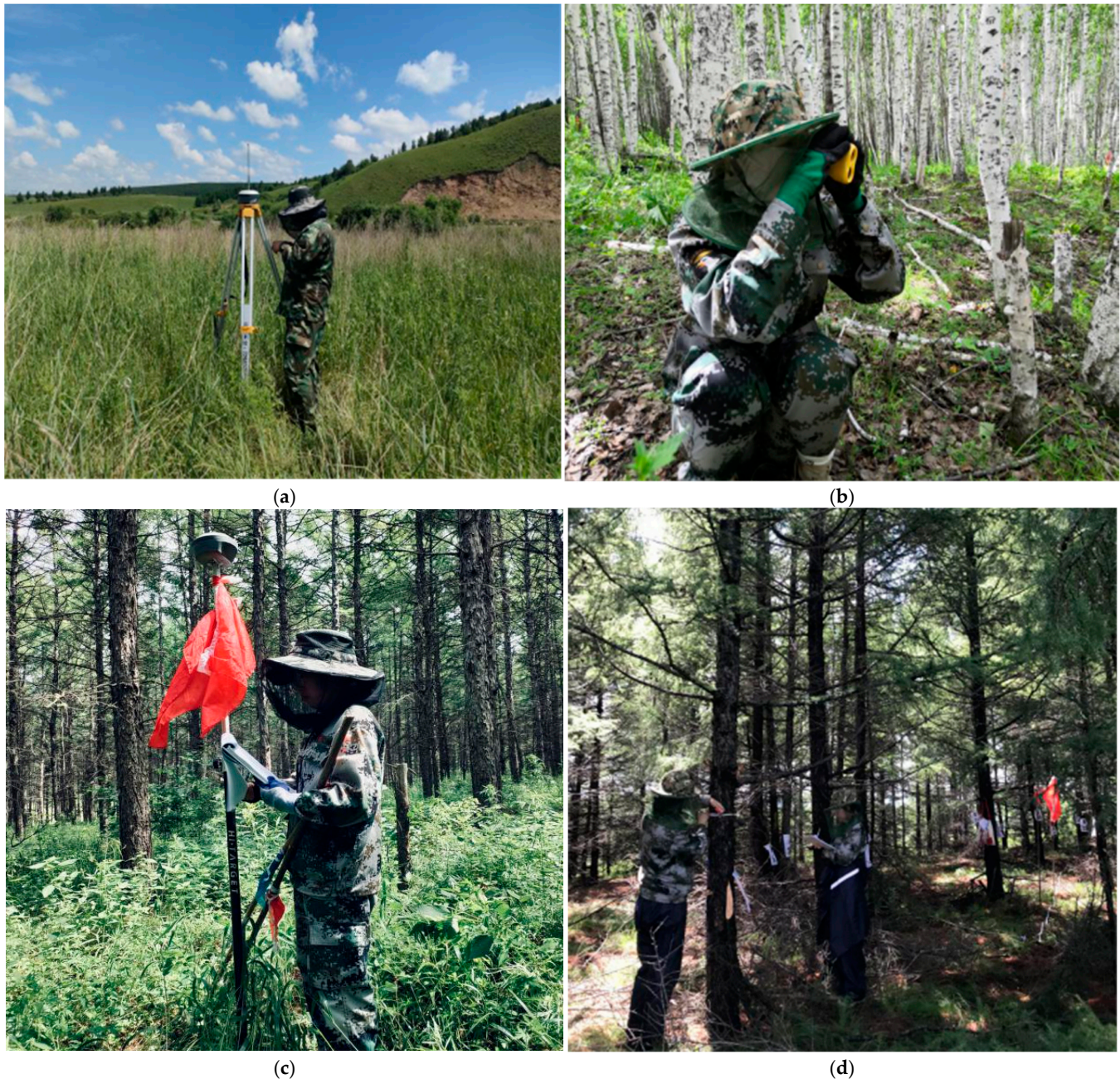
Figure 2. Parameter measurements in the study area: (a) Setup of base stations. (b) Tree height measurement. (c) Obtaining the coordinates. (d) DBH measurement and recording.
