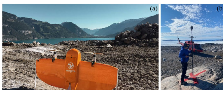
Figure 3. WingtraOne UAV (a) and survey of the RTK roving stations (b).
