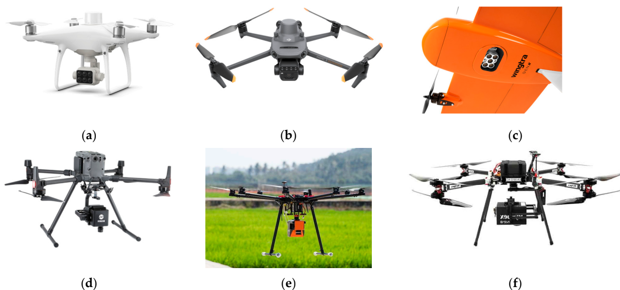
Figure 1. UAV systems with multispectral and hyperspectral sensors. (a) DJI P4 Multispectral, (b) DJI Mavic 3 Multispectral, (c) Wingtra GEN II, (d) Matrice 300 RTK, (e) SPECIM AFX SERIES, (f) HySpex Mjolnir.
