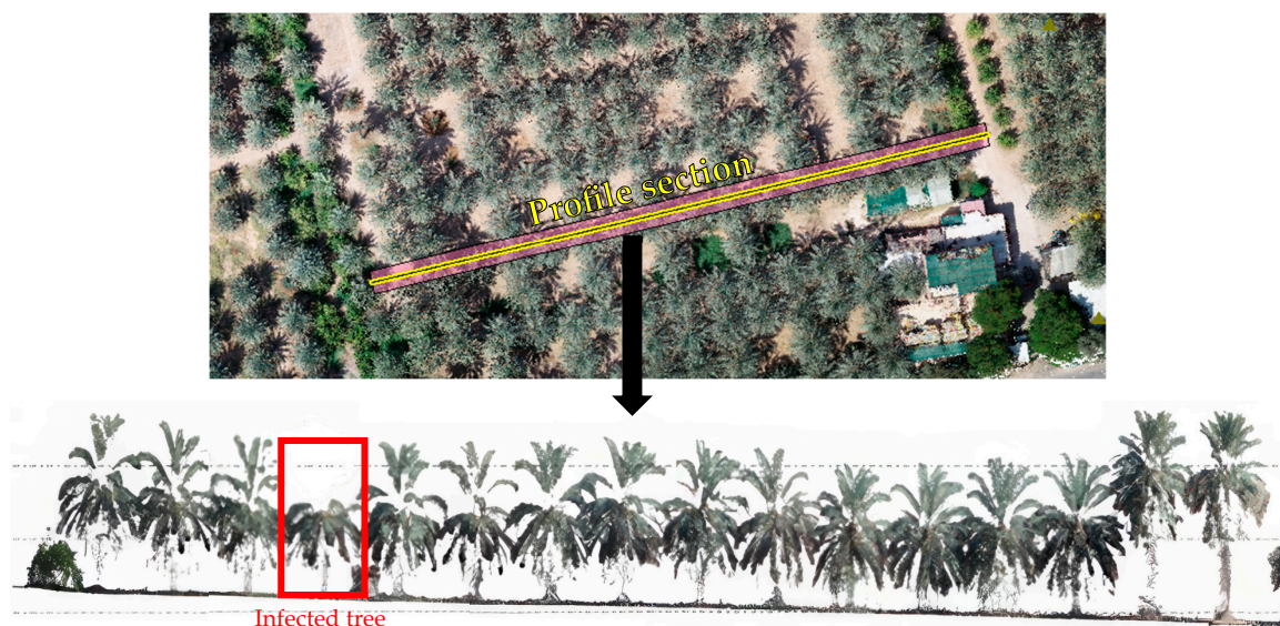
Figure 5. A profile section taken from a LiDAR point cloud of a palm tree farm shows a possible infected tree with missing fronds.
