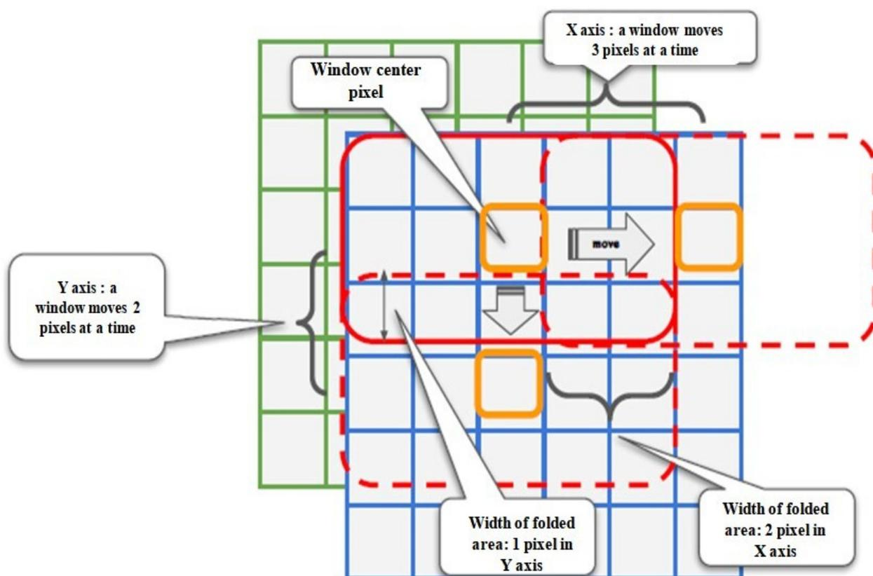
**Figure 3.** Schematic diagram of moving window method.
