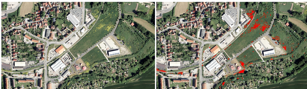
Figure 5. DOP captured in May near Ebeleben in Thuringia depicting occurrences of Bunias orientalis visible as yellow spots on the left side and highlighted in red after the automated segmentation classification on the right side.
