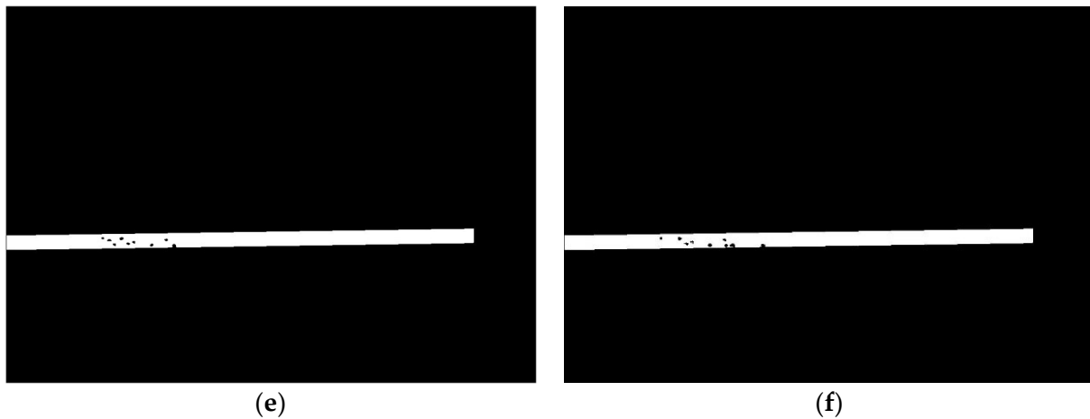
Figure 11. Test Image #6: (a) original image; (b) the result of the proposed runway extraction method marked with red box; (c) the result of the proposed crater extraction method marked with red circles; (d) the result of the method [32] marked with red circles; (e) the binary result of the proposed method; (f) ground truth of runway and craters.
