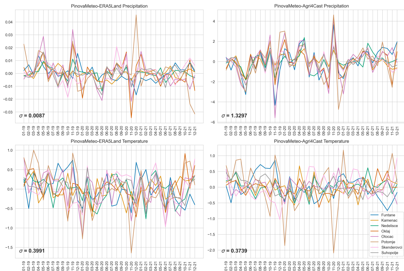
Figure 4. Residuals of monthly mean temperature and precipitation between data source PinovaMeteo (ground-based) and two model-based data sources Era5-Land and Agri4Cast. Standard deviations are shown within plots in bold.
