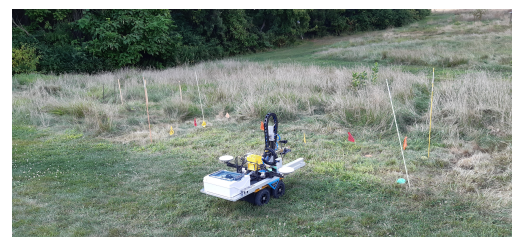
(b) Demining robot scanning test field.
