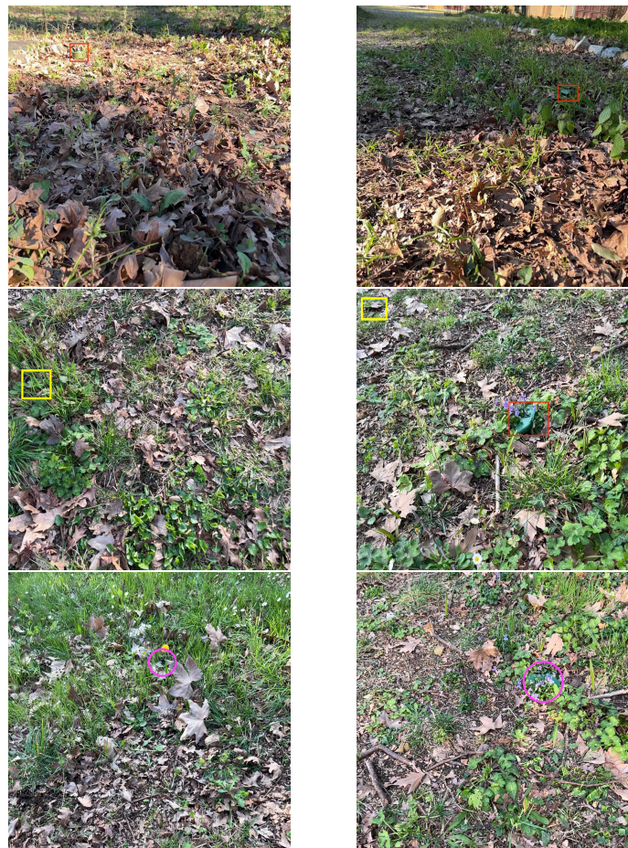
Figure 7. Example of correct (top), wrong (middle), and missing (bottom) detection for “starfish” (left) and “butterfly” (right). Detected objects are shown with a red rectangle, wrongly detected background for landmines in yellow, and missed landmines circled in purple.
