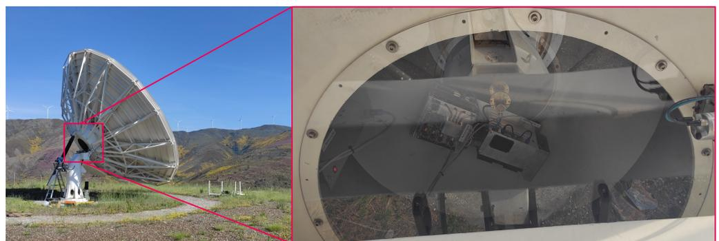
**Figure 1.** Antenna located in PASO, with the radar system inside the hub.
