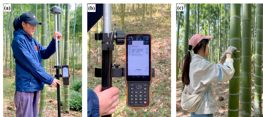
Figure 3. Ground survey: (a,b) RTK positioning of sample plots (c) single-tree diameter at breast height measurement.
