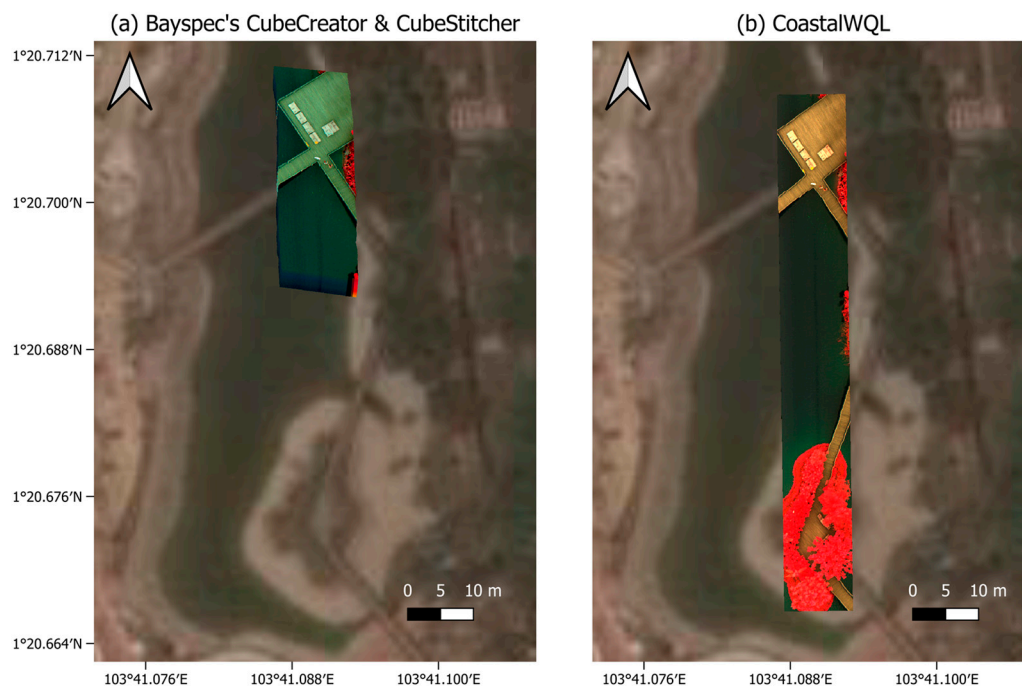
Figure A12. Mosaicked image output from Bayspec's CubeCreator and CubeStitcher, in comparison with the output from CoastalWQL (Notes: the mosaicked image outputs from CubeCreator were not successfully stitched in CubeStitcher and Agisoft Metashape to form an image line due to lack of tie points and distortions at the image edges).
