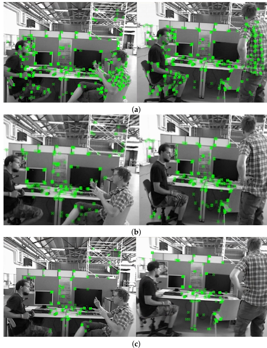
Figure 10. Elimination of dynamic feature points in images by the three systems; the images on the left came from the sitting sequence, while the images on the right came from the walking sequence. (a) ORB-SLAM3. (b) DynaSLAM. (c) Transformation matrix estimation.
