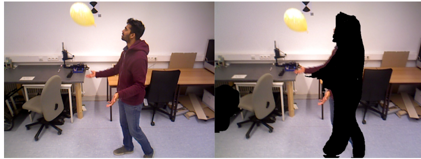
Figure 14. DynaSLAM's utilization of Mask R-CNN for the semantic segmentation of dynamic objects in b_balloon.
