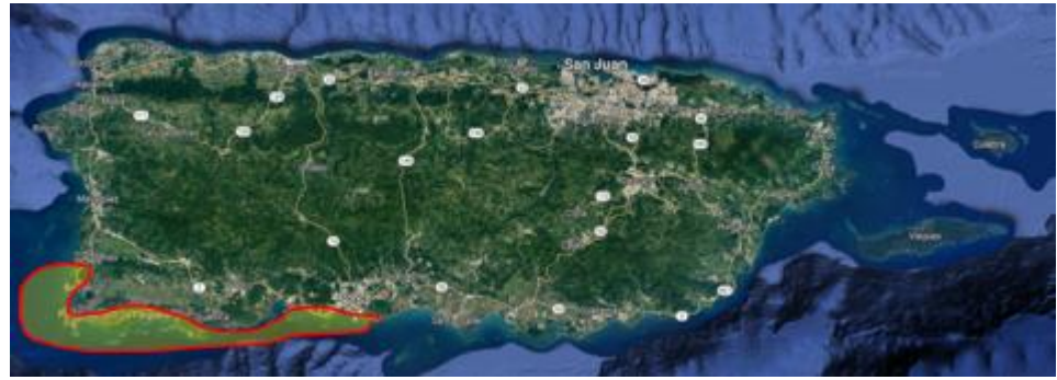
Figure 32. SDB of the entire local region in Puerto Rico after fine-tuning using partially available TBDEM. The known TBDEM area is marked as a red-colored boundary.
