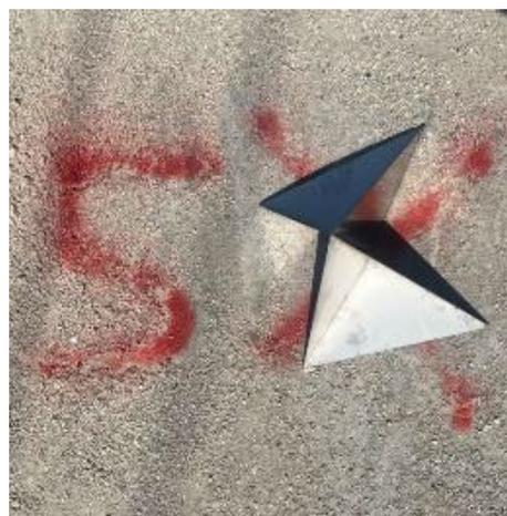
Figure 19. The No.5 GCP (0.3 m calibrator).
