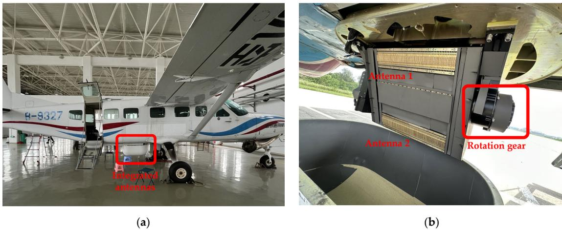
**Figure 3.** Antenna structure: (a) Installation diagram (red frame is mounted antenna) and (b) antenna structure details (red box for rotating mechanism).
