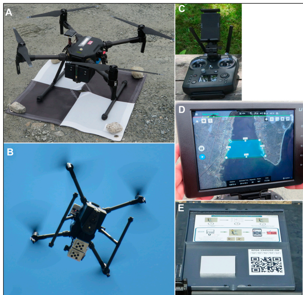
Figure 2. Photographs of (A) DJI Matrice V2 aerial drone and MicaSense Downwelling Light Sensor (DLS), (B) airborne drone showing the MicaSense Dual Camera System, (C) DJI Cendence remote controller, (D) DJI CrystalSky tablet with DJI Pilot software, and (E) Spectralon panel (RP04-1949202-OB).
