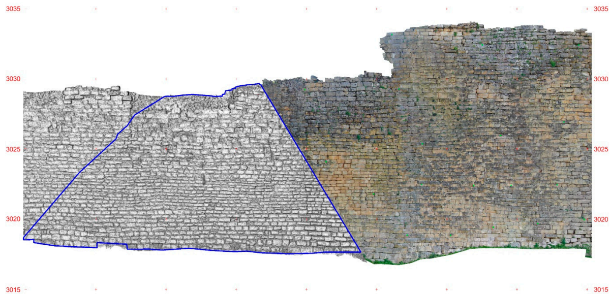
Figure 18. Sample of the fusion of digital photogrammetry and TLS data at the southeastern corner of La Fortaleza’s perimeter wall. Blue lines—overlap between TLS and photogrammetric projects; green crosses—ground control points for photogrammetric project. TLS 3D point cloud data from Kucera, VanValkenburgh, and Rojas. Elaborated by Kościuk.
