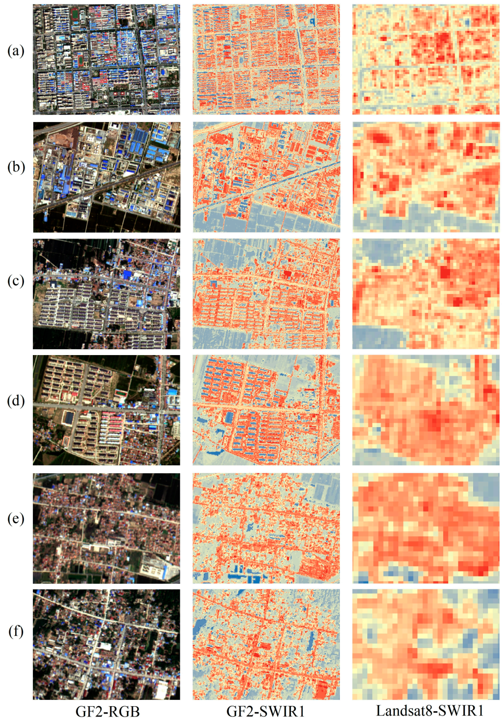
Figure 4. Comparisons of downscaled and original SWIR1 bands. RGB means the red, green, and blue channels for image displaying. (a,b) towns; (c,d) allocation communities; (e,f) villages.
