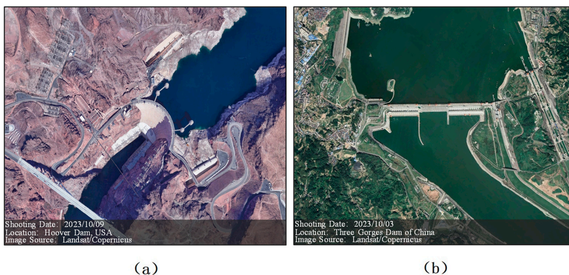
Figure 4. Dams in Remotely sensed Images (Image Source: Landsat/Copernicus), ((a) depicts the arch-shaped Hoover Dam in the U.S.; (b) showcases the straight-line structure of the Three Gorges Dam in China).
