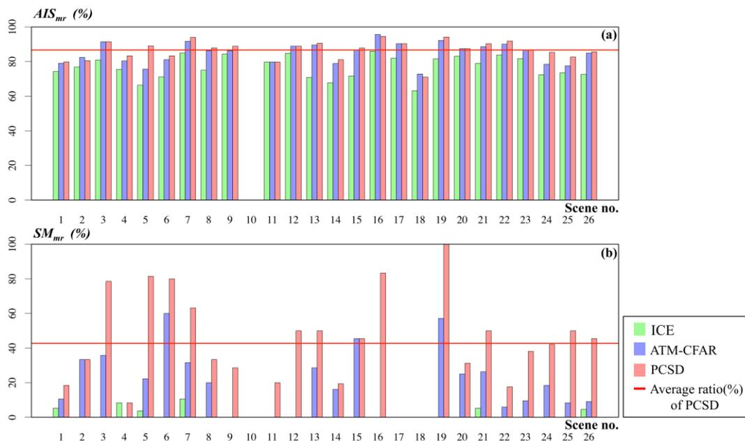
**Figure 14.** Comparison graph illustrating the performance of three different ship detection models for the year 2022 (26 scenes). (a) Represents the matching ratio for AIS-ships; (b) Displays the matching ratio for the small ships. Here, AIS = Automatic Identification System, SM = Small ships, ICE = Image Contrast Enhancement, ATM-CFAR = ATM-Constant False Alarm Rate.
