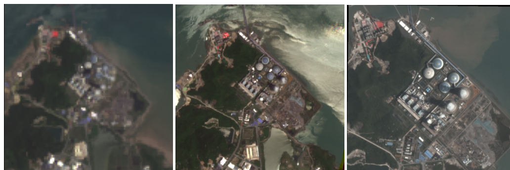
Figure 3. The Ninghai power station in China as seen from Landsat 8 at 30 m spatial resolution ( left ), Sentinel-2 at 10 m spatial resolution ( center ), and PlanetScope at 3 m spatial resolution ( right ). These images only represent the visible bands (red, green, and blue).
