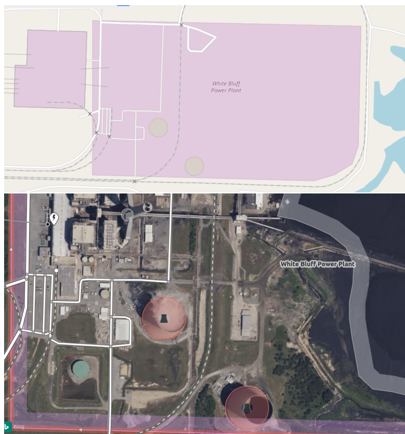
Figure A1. White bluff power station as shown on OpenStreetMap ( top ) and in OpenStreetMap edit mode ( bottom ). We used this aerial imagery to annotate the locations of FGD flue stacks (translucent white circle) and NDT cooling towers (red circles).
