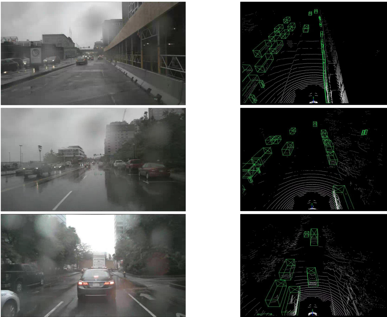
Figure 9. Detection results of the proposed method in rainy conditions. The green boxes represent the predicted boxes by algorithm.
