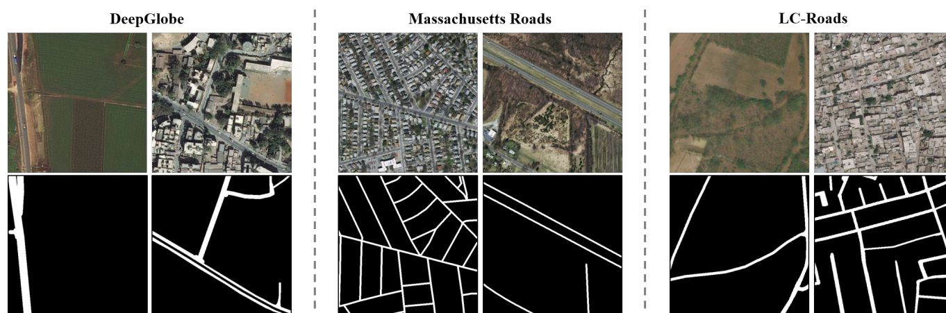
Figure 2. Example images and ground truth from the DeepGlobe dataset, the Massachusetts Roads dataset, and our LC-Roads dataset. There are two classes in the ground truth: background (black) and road (white).
