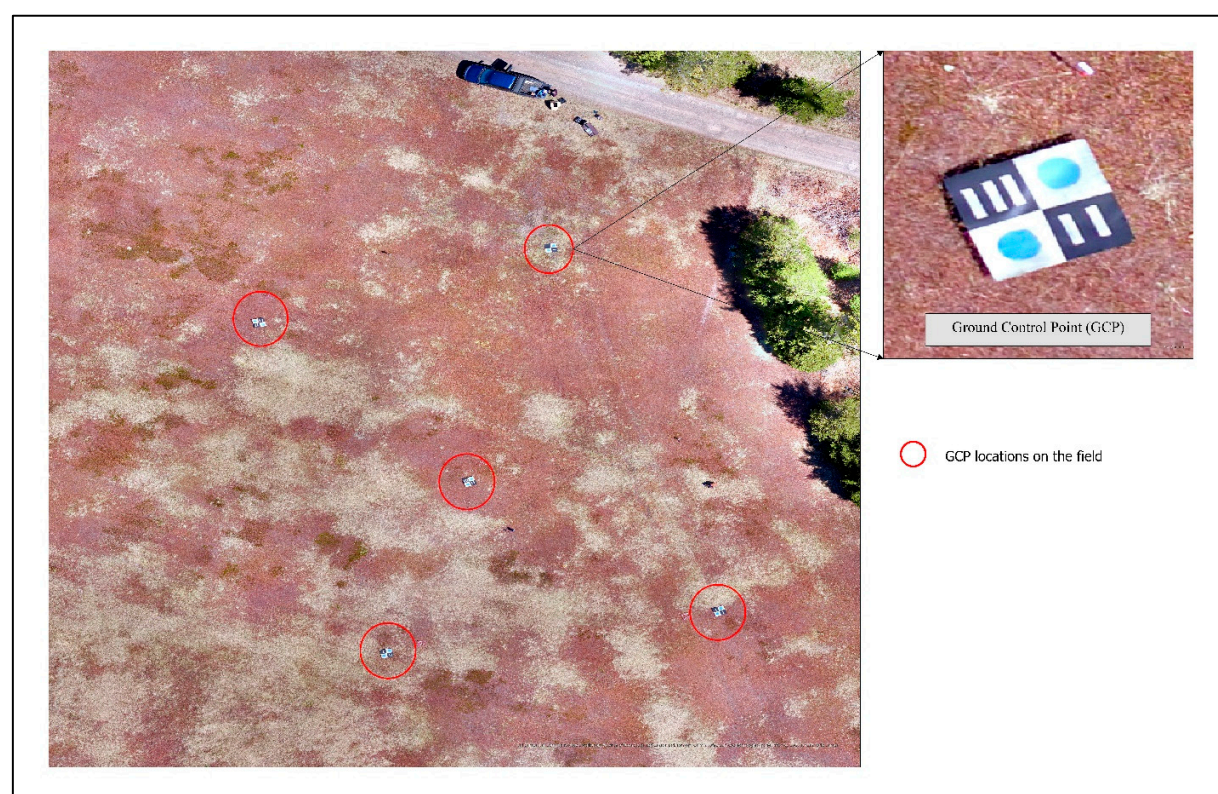
Figure S1. Ground Control Point deployed at the Kemptown Trial site before aerial surveys.
