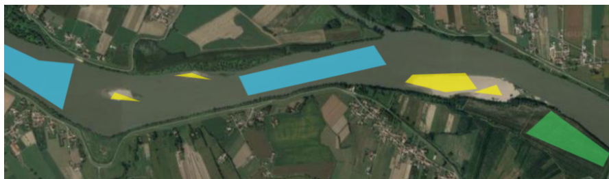
Figure 4. Polygons, manually extracted in GEE, and evaluated in Random Forest Algorithm. In the image, green polygons is for the vegetation, yellow ones for the sediments, and blue for the water.
