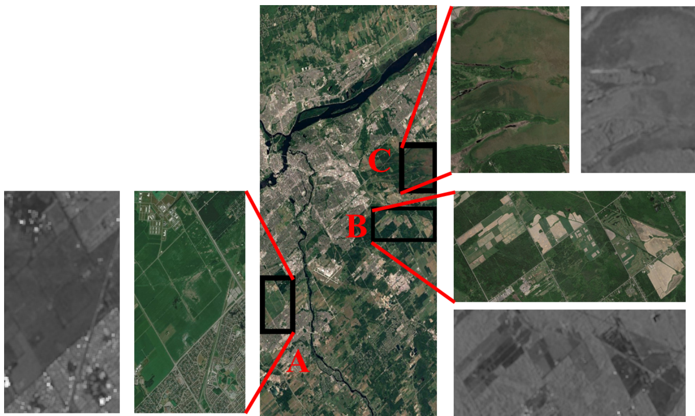
Figure 5. The Google Earth image of the test scene with three regions of interest along with their corresponding |S_{RH}|^2 . Regions A and B primarily consist of urban, farm and forest classes, while Region C displays both forest and farm classes.
