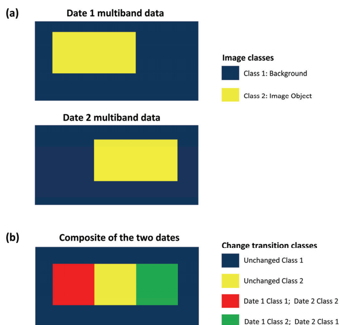
Figure 2. Schematic outline of the process of construction of a two-class, two-band simulated data set.
