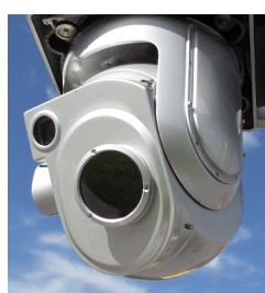
Figure 1. An example of a gimballed sensor system with infrared and video sensors. The gimbal has two actuated axis pan (azimuth) and tilt (elevation) that decides the pointing direction of the sensors. The sensor system is assumed to be mounted on a UAV platform.
