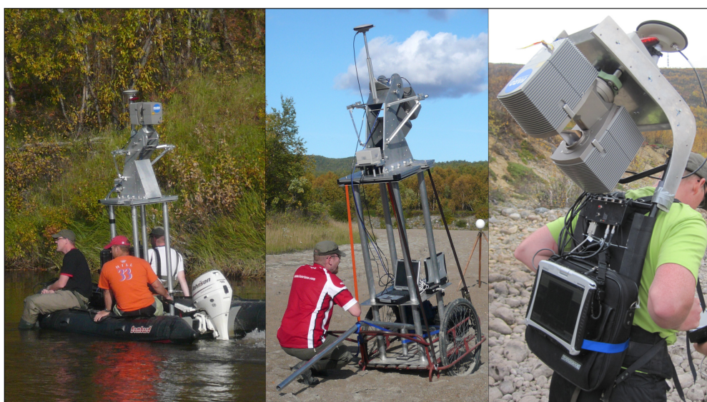
Figure 1. Different setups for the FGI ROAMER mobile mapping system: BoMMS (left); CartMMS (centre); Akhka (right).
