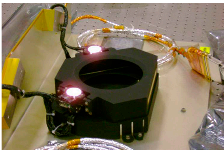
Figure 5. The two stim lamp assemblies mounted to the aperture baffle ( left ); a schematic of the stim lamp assemblies showing the six bulbs and the monitoring diode (which looks at the stim lamp diffuser) ( right ).
