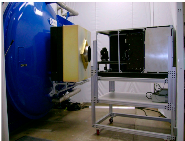
Figure 18. The spectral measurement assembly in front of the sphere. The gold box attached to the chamber is a light shade.
