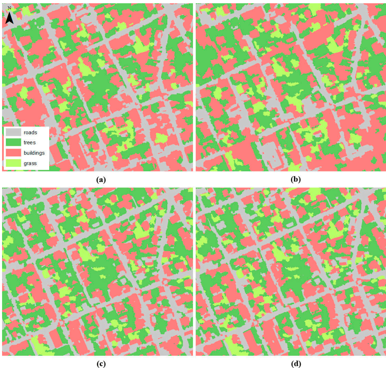
Figure 10. The final classification image for all four classifiers related to the 8-band classification results presented in Table 4: (a) k -NN; (b) SVM; (c) the two-sample Kolmogorov-Smirnov statistics based classifier; (d) the Student's t -test statistics based classifier.
