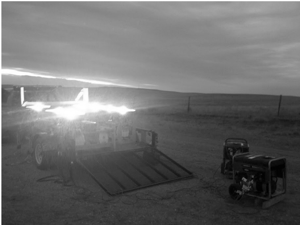
Figure 2. Seven (1000 watt) high pressure sodium lights in the utility trailer and the two generators used to power the lights in the field.
