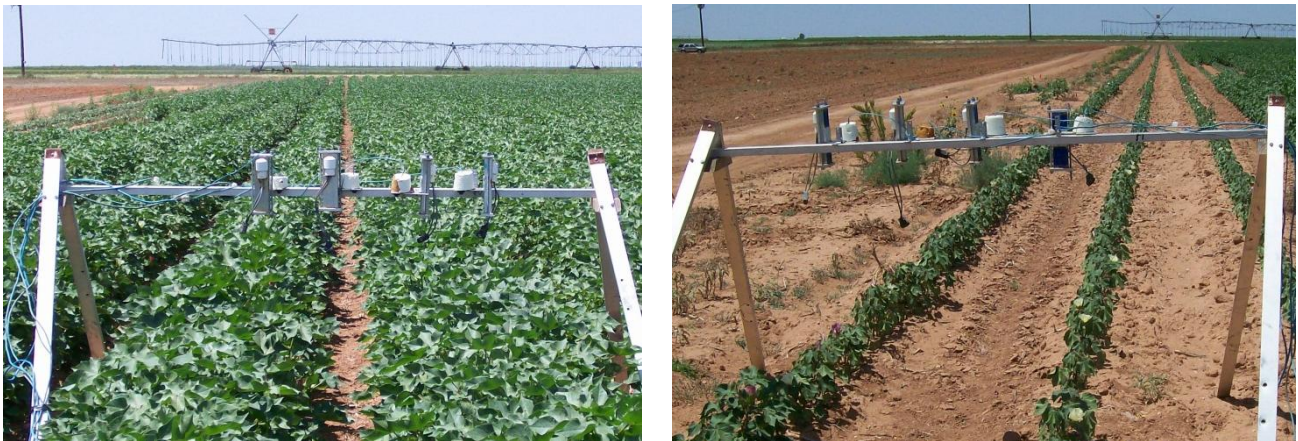
Figure 2. Array of sensors used to monitor surface temperature ( T_s ): (left) high irrigation treatment; (right) dryland treatment.
