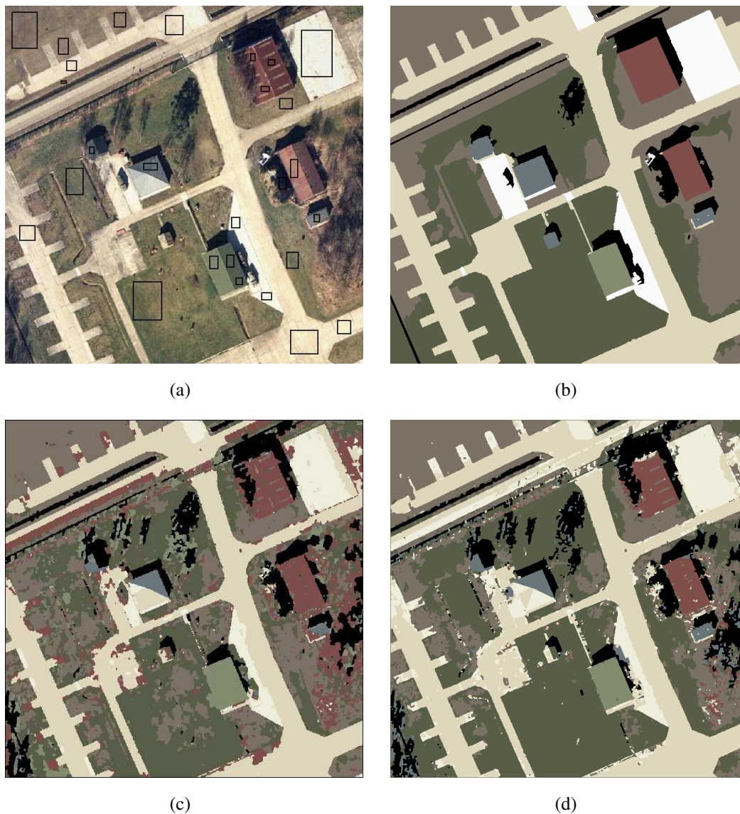
Figure 13. The proposed multi-scale CRF exhibits superior classification results compared with MRF for the airborne image. (a) Training samples. (b) Testing samples. (c) Multi-scale MRF (MRAT) [3]. (d) Proposed multi-scale CRF (A-MRAT).
