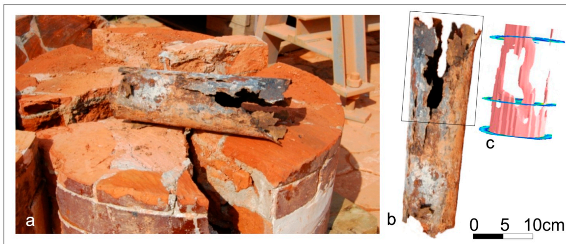
Figure 11. (a) Section of the column after the compression test and (b) the metallic tube extracted, compared to (c) 3D radar imaging from isoamplitudes after a cylindrical interpolation.
