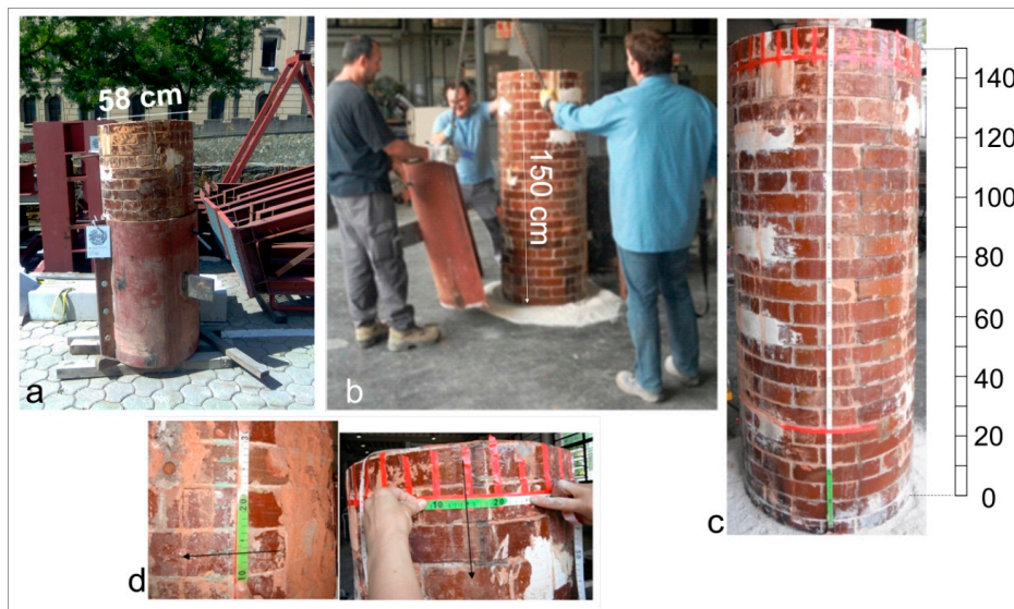
Figure 2. Preparing the specimen for the test. (a) The column with the metallic jacket; (b) the test site; (c) the column prepared to be tested; (d) the distance between horizontal and vertical radar lines.
