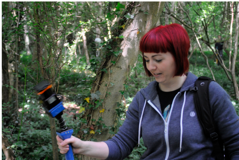
Figure 1. ZEB1 handheld mobile laser scanner in operation for forest mapping.
