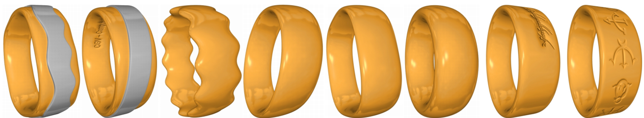
Figure 2. The presented generative description is able to produce a large variety of wedding rings. Features, like engravings, recesses, different materials, unusual forms and gems, can be created and customized.
