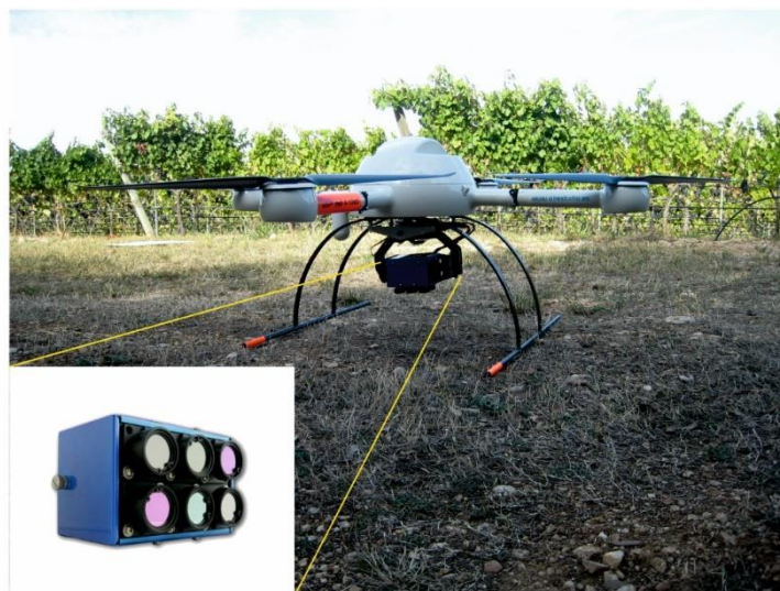
Figure 2. Multispectral camera mounted on the RPAS Md4-1000 and detail of the multiple camera array.
