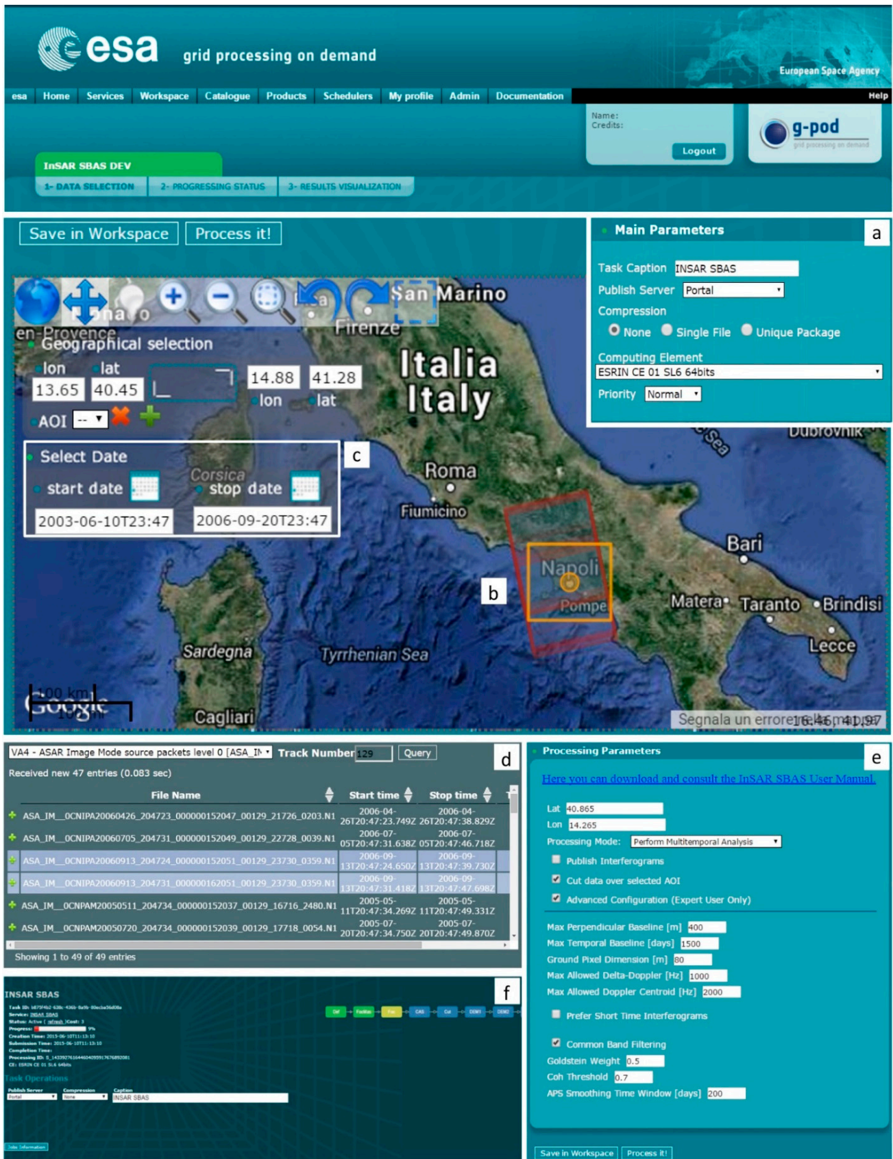
Figure 2. P-SBAS tool web portal. (a) Main processing Parameters window, (b) geographic map client for the AoI and data selection, (c) investigated time interval selection, (d) SAR data catalogue query, (e) interferometric processing parameters window, and (f) job status monitoring.
