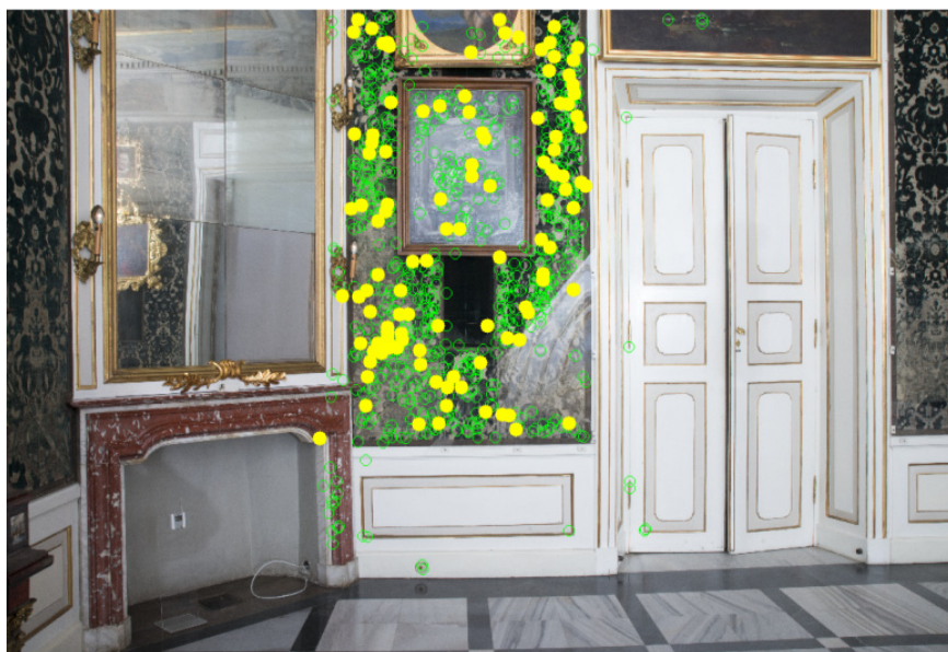
Figure 22. Example of utilized image with points used for orientation (control points, in green) and yellow “o”—check points.
