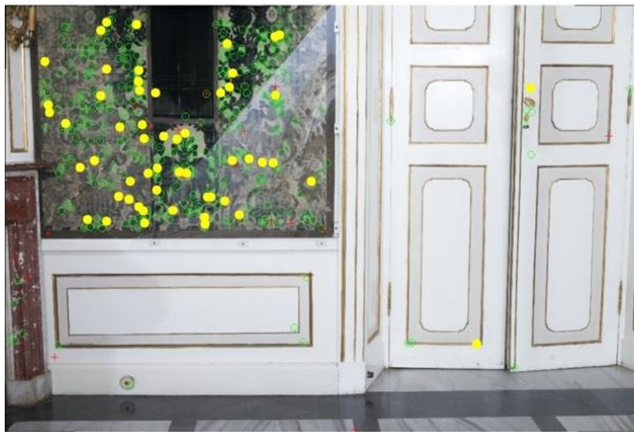
Figure 19. Distribution of points detected in the single image (from a group) and in the orthoimage: green “o”—control points; red “+”—wrong matched points; yellow “o”—check points.
