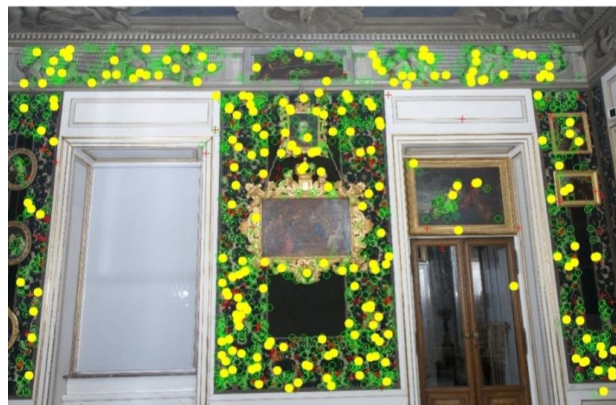
Figure 17. Example of utilized image with control points in green and points eliminated from the adjustment process in red; a yellow “o”—a check point.
