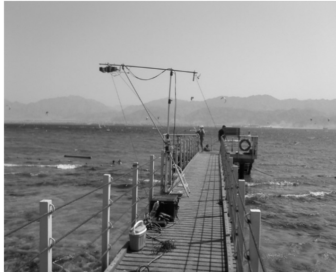
Figure 1. The hyperspectral camera setup over the jetty. The jetty is built about 1.5 m above the reef table. The camera construction was made so it took near nadir images, 3 m above the jetty. Ropes were used to stabilise the entire construction against wind.
