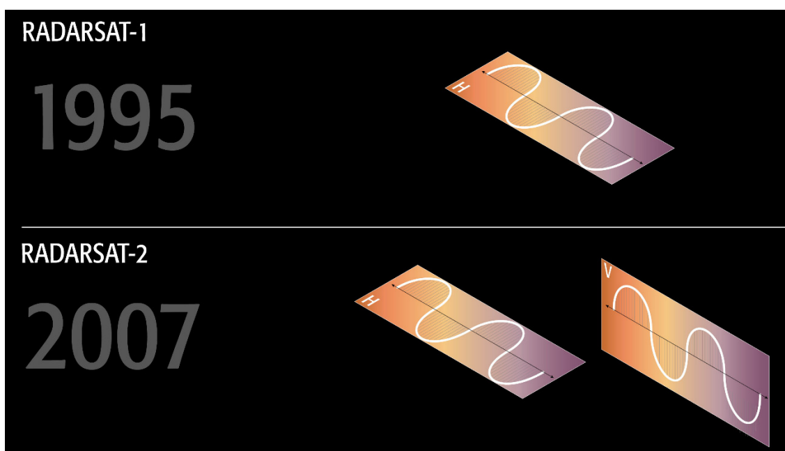
Figure 1. A comparison of how RADARSAT-1 and RADARSAT-2 transmit and receive radar waves. RADARSAT-1 transmits and receives radar waves horizontally to the target on the ground. RADARSAT-2 can transmit and receive radar waves in both the horizontal and vertical polarization planes, allowing calculation of the phase. Reproduced by permission of/ or Courtesy of MacDonald, Dettwiler and Associates Ltd.
