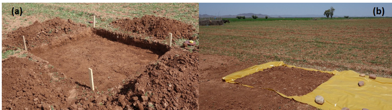
Figure 2. Illustration of the dry soil plot in the R3 perimeter. (a) The pit was dug at a 15-cm depth and (b) the soil plot was kept fully dry by covering it with a plastic sheeting in between experiments.
