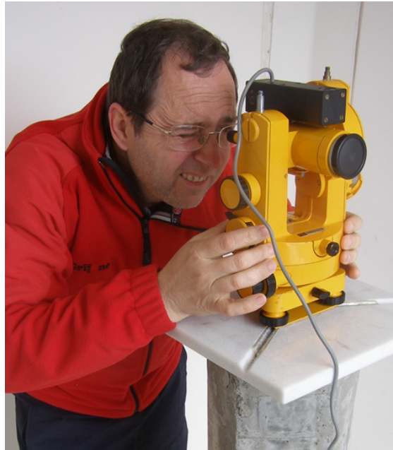
Figure 2. The manual declination and inclination (D/I) fluxgate theodolite being manipulated by a specialist. More details about the sensor can be found in [9].
