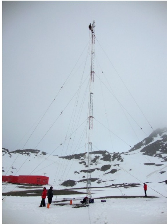
Figure 5. The vertical incidence ionospheric sounder (VIS) installed at the ASJI is the Advanced Ionospheric Sounder (AIS) developed by the Istituto Nazionale di Geofisica e Vulcanologia (INGV) of Rome, Italy. For more details about the ionosonde, see [12].
