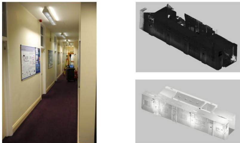
Figure 5. Image of corridor ( left ) and resulting point cloud data collected with a Viامتري Indoor Mobile Mapping System ( top right ) and Faro Focus 3D S ( bottom right ).
