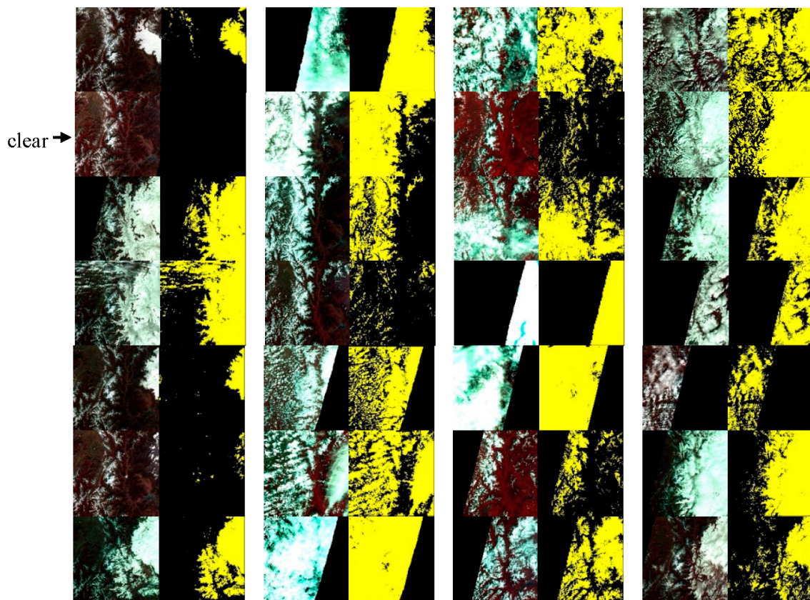
Figure 8. Examples of performance of the proposed algorithm for 150 \text{ km} \times 150 \text{ km} Mt. Gongga area for the middle month of each season of the year 2011. The standard seasonal definition for the Northern Hemisphere adopted by the climate modeling community is used, where spring is defined by the months March to May. False color composited images with bands 4, 3, and 2 in red, green and blue, respectively, are shown on the left, and cloud masks are shown on the right with yellow color.
