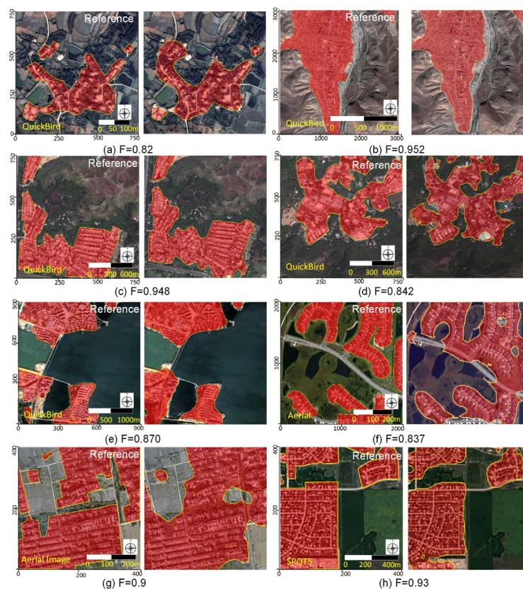
Figure 16. Built-up area detection using different images and different scenes with the proposed method. (a,b) Built-up area detection over hilly areas using QuickBird images with a resolution of 0.6 m/pixel; 750 \times 750 and 2961 \times 3108 pixels; (c,d) Built-up area detection over mountainous areas using QuickBird images with a resolution of 2.4 m/pixel, 750 \times 750 and 750 \times 750 pixels; (e–h) The detection results over flat areas using QuickBird ( 2.4 m/pixel, 900 \times 900 pixels), aerial ( 0.32 m/pixel, 2001 \times 2001 pixels, and 1 m/pixel, 400 \times 400 pixels), and SPOT-5 ( 2.5 m/pixel, 400 \times 400 pixels) images, respectively.
