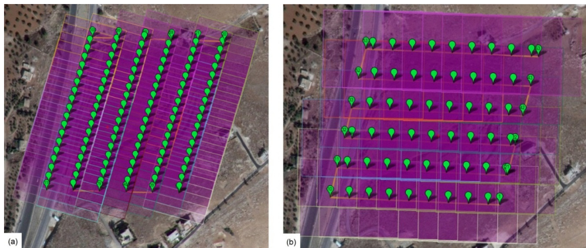
Figure 7. Graphical interface of the image capturing mission flight plan designed to cover the area of interest: (a) north-south flight path and (b) east-west flight path.
