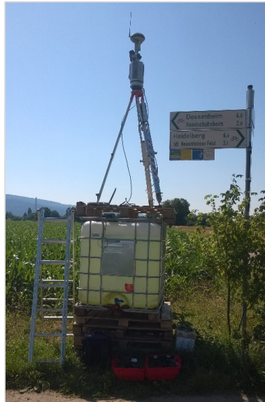
Figure 1. Scanner set up on barrel for elevated scanning at a height of 3.6 m, located at one edge of the monitored maize field.
