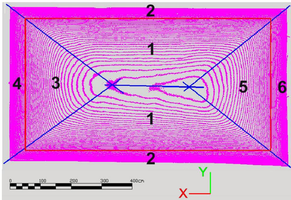
**Figure 3.** Discontinuity directions and vault areas (bottom view).
