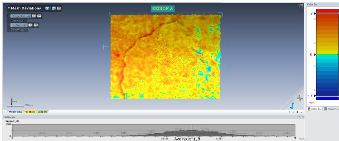
Figure 14. Region A: total plaster collapse borders.
