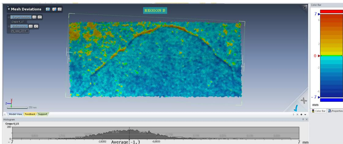
Figure 15. Region B: total plaster collapse borders.
