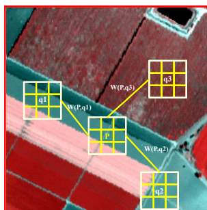
Figure 3. The basic principle of the nonlocal means model.
